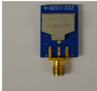
(c) Patch Antenna Working at 4.5 GHz
